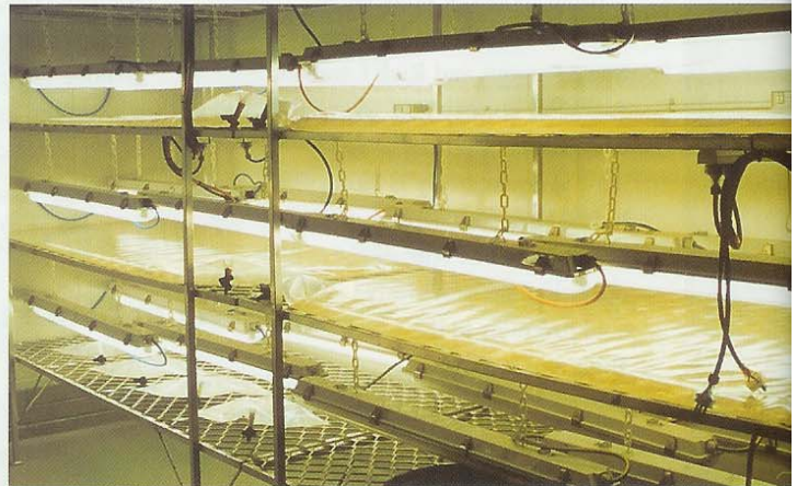
Large plastic algal culture bags are used to grow the Navicula diatom under artificial lighting.
